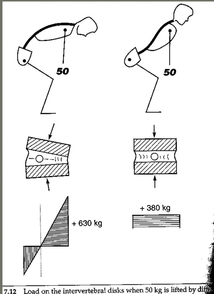
7.12 Load on the intervertebral disks when 50 kg is lifted by different techniques.
